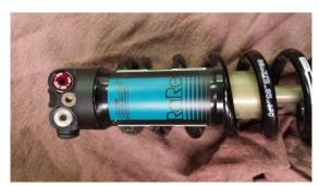
Red adjuster = High Speed Compression Silver adjuster = Low Speed Compression
